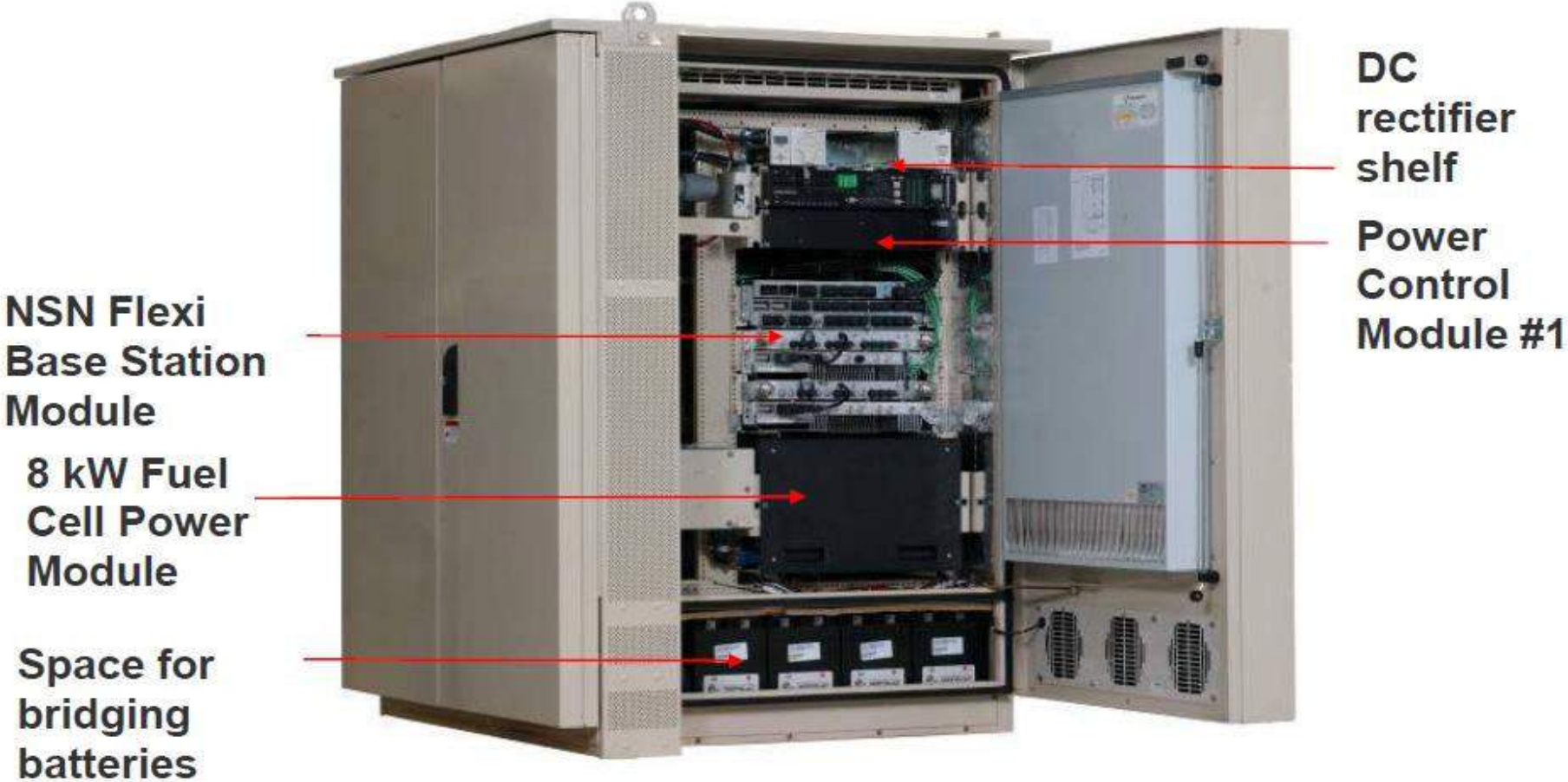
Cabinet dimensions: W 45" (1143mm) x D 52" (1321mm) x H 63" (1600mm)
