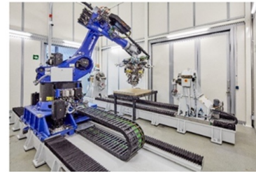
automatic fiber placement (AFP) process
