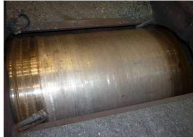
The SMS Group roller with our mineral coating (42 month of using) / 3 375 000 tons
