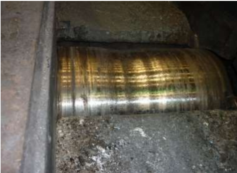
The SMS Group roller without any coating (8 month of using) / 600 000 tons
